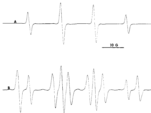
Figure 3. Effect of ethanol on hydroxyl radical trapping by DMPO. (A) ESR spectra produced by UV photolysis of a 0.6% H_2O_2 pH 7.4 phosphate buffer containing 0.09 M DMPO. The spectrum is of DMPO-OH, A_N = A_H = 14.9 G. (B) Conditions were the same as those for A, except that 0.33 M ethanol was present and the instrument gain setting was higher. Spectra are a combination of the hydroxyl and \alpha -hydroxyethyl radical adducts. For the \alpha -hydroxyethyl adduct, A_N = 15.8 and A_H = 22.8 G.
